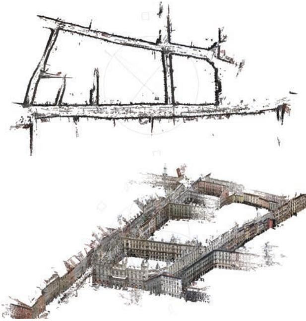
Figure 4: Sparse reconstruction data set. For better visualization a quasi-dense point cloud was created using [7].
