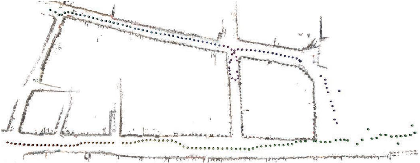
Figure 12: The path of panoramic images through the reconstruction. The camera positions are drawn as color coded cylinders, starting from the bottom left area and ending in the upper left area. Some localization results fail in the upper right area due to missing parts in our reconstruction.
