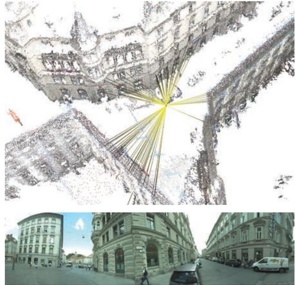
Figure 1: Localization result given the panoramic image shown at the bottom.
