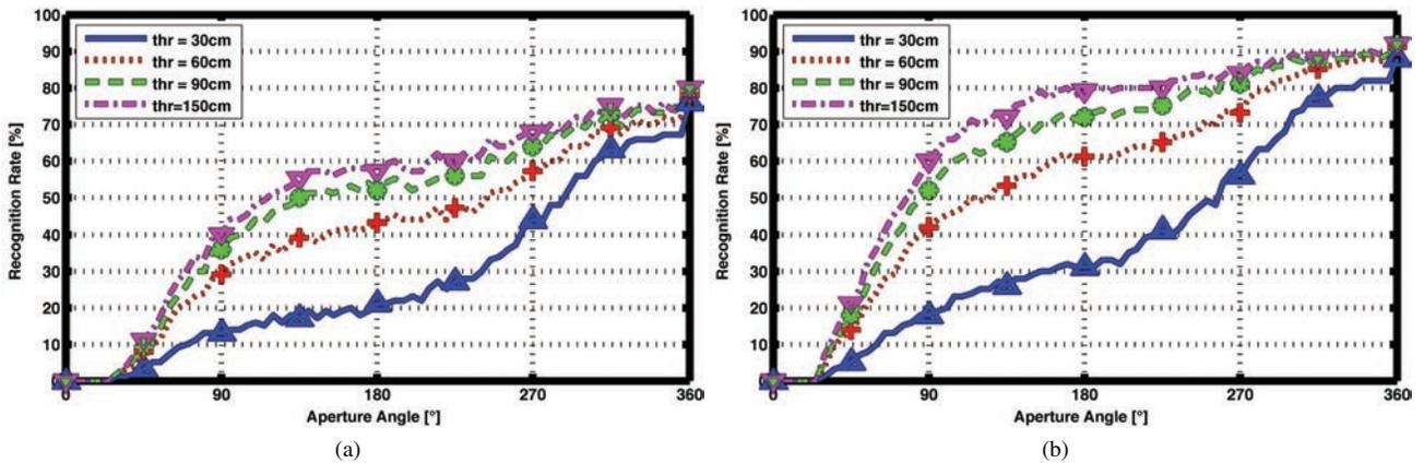
Figure 10: Success Rate for different thresholds applied on the translation error and manually selected starting points. The tree-based matching results are depicted in (a), the exhaustive matching based results are shown in (b). Compared to Figure 9, for small FOV higher success rates are achieved under a relaxed accuracy constraint.
