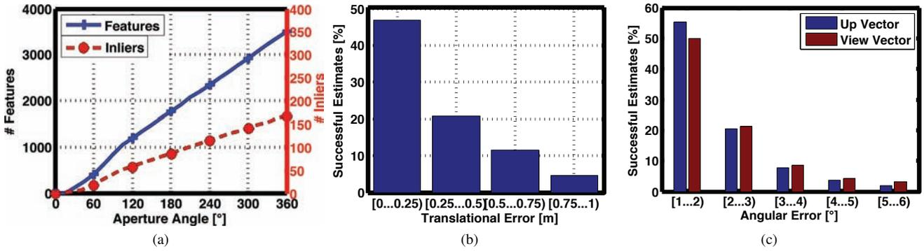
Figure 8: Localization Performance for a varying FOV. (a) The average number of inliers is approximately 5% of the features and increases linearly with the number of features detected in the entire image. (b) For around 84% of all successfully determined poses, the positional error is below 1m. (c) For around 88% of all successfully determined poses, the rotational error for both the view vector and the upvector is below 5 degrees.
