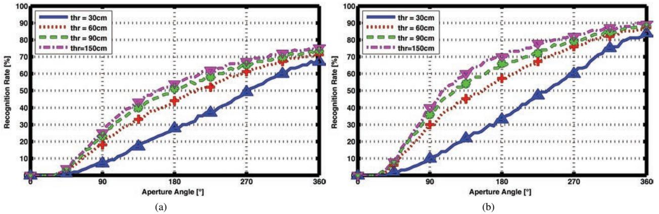
Figure 9: Success Rate for different thresholds applied on the translation error and random starting points. In (a) the tree-based matching is depicted, while in (b) the exhaustive matching based results are shown. The results of the tree-based matching are 5-10% worse than the results of the exhaustive matching approach.
