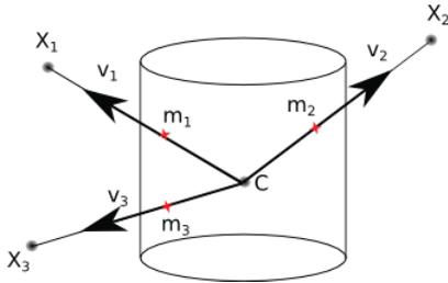
Figure 7: The geometry of the  $P3P$  problem for panoramic camera models is the same as for pinhole models. The law of cosines relates the unknown distances of 3D points and the camera center  $x_i = \|C - X_i\|$  with the pairwise angles  $\angle(v_i, v_j)$  of the image measurement rays.
