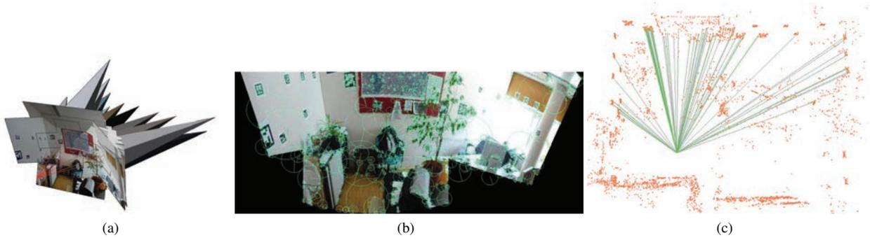
Figure 6: Extending the field of view illustration. (a) Relative orientation of images with the same projection center. (b) Feature points are extracted in the blended cylinder projection of the images. (c) Inlier feature matches for the panoramic image after robust pose estimation against a small office test database, the lines connect the center of projection with the matched database points.
