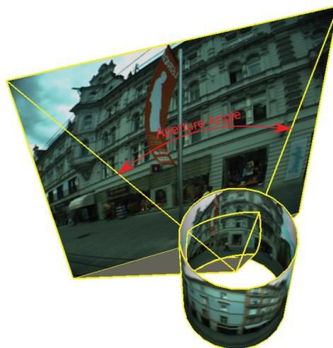
Figure 3: Panoramic Mapping of the environment onto a cylindrical surface. We use the term *angular aperture* to describe the FOV of a camera.
