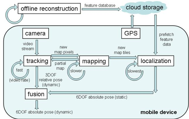
Figure 2: Overview of the localization system – three activities are performed simultaneously: orientation tracking, mapping of a panoramic image, and localization of the panoramic image relative to a large-scale 3D reconstruction. The results are combined into a 6DOF absolute pose measurement.
